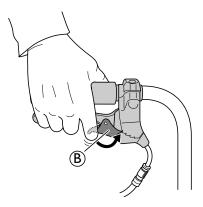
Pull the brake handle upwards and push the lock catch ® downwards to lock the brake.
