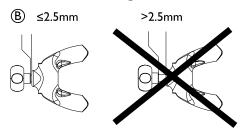
Make sure that the hand wheel for the push handle (a) fits the hole in the tubes. If the threaded tap of the hand wheel (b) is more than app. 2.5 mm visible, the position is wrong. Lower or raise the push handle to get the hand wheel in the correct position.
