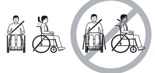
Attach the 3-point passenger restraint system referring to the user manual supplied with your 3-point restraint system.
