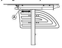
Slide the half tray (A) forwards or backwards to adjust to the required depth.
