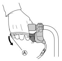
Move the brake handle (A) to release the lock catch.
