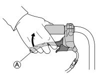
Pull both brake handles upwards to engage the brake.
