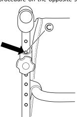
In order to lock the position of the push handle, the nearest upper hole © should be visible, just as shown on the picture above.
