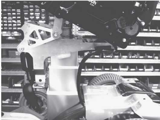
Fig. 11-7 Lifter column completely extended
