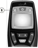
1. Press the direction indicator left key (1) for more than 3 seconds.
