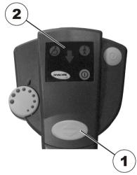
You can set whether the wheelchair should travel forwards or backwards by pressing the switchover button for forwards or reverse gear (1). If reverse gear has been selected, the arrow (2) illuminates.
