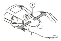
When reversing, make sure you know whether the wheelchair has direct or indirect steering so that you know in which direction you have to steer, and then in which direction the wheelchair will actually travel. You should initially get used to the IDC attendant control in stages so that no hazards are posed for the wheelchair driver or others.
