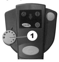
The maximum speed of the wheelchair can be set by the user to match his personal requirements and the surrounding conditions. The current maximum speed set is displayed on the wheelchair speed display and can also be preset there. You can carry out further fine adjustments to the maximum speed on the IDC using the speed potentiometer (I). In addition, the speed increases the more the drive button is pressed.
