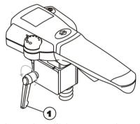
Loosen the clamping lever (I) (rotates several times!) and pull the control unit out of the wheelchair bracket.
