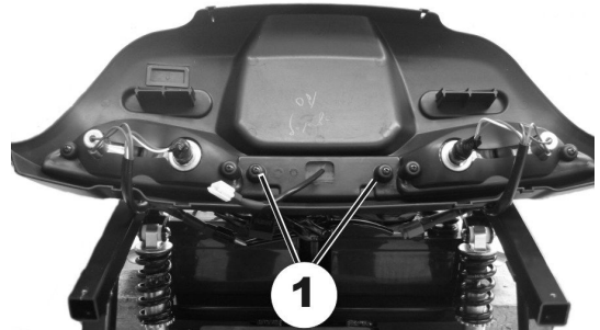
Remove screws (1) on brake light.
